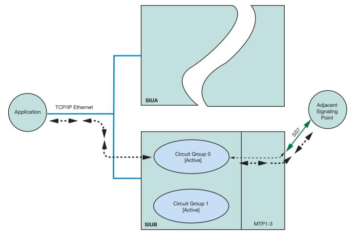
Figure 12. Routing Following Failure of SIUA
